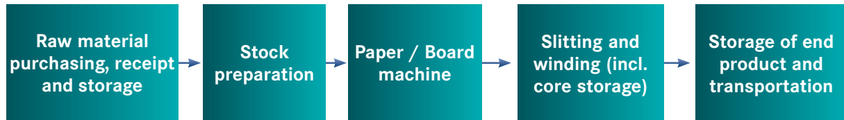
Figure 5 – Flow Chart for Papermaking Process
